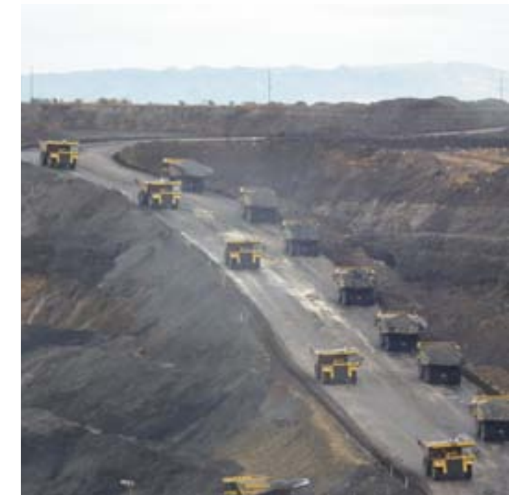
Moving equipment with headlights on at all times while maintaining safe distance of 30 meters downhill and uphill.
